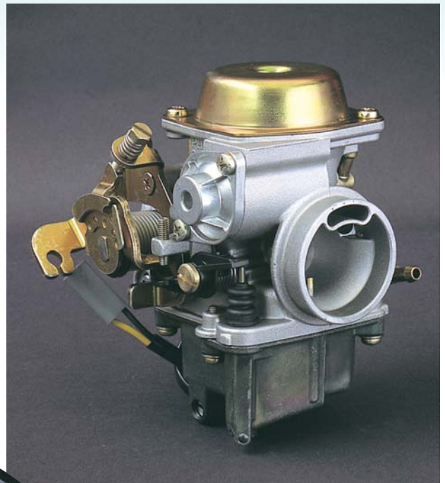
Three views of the Dell'Orto vacuum carburetor: we can see the piston accelerator pump assembled in the float chamber and the automatic starting system with the compact type actuator shorter than the traditional ones.
